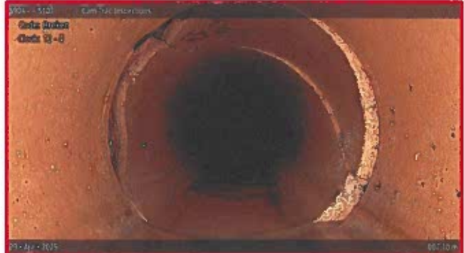
[Grade 4] Broken at 007.10 m, 8 - 4 o'clock
