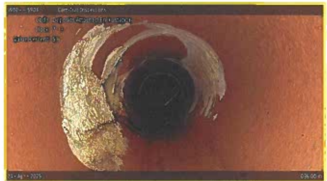
[Grade 2] Deposits Attached Encrustation at 036.00 m, 7 - 3 o'clock
