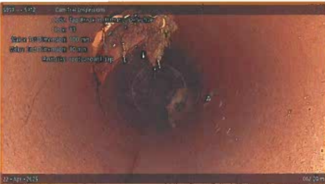
[Grade 3] Tap Break-in/Hammer Defective at 062.20 m, 11 o'clock | roots around tap
