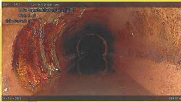
[Grade 2] Deposits Attached Encrustation at 030.80 m, 6 - 11 o'clock
