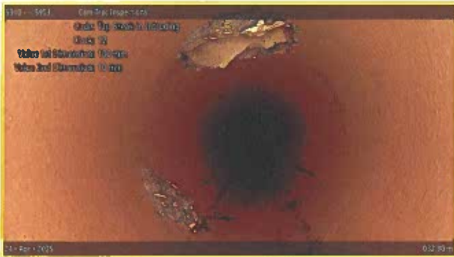
[Grade 2] Tap Break-in Intruding at 032.90 m, 12 o'clock
