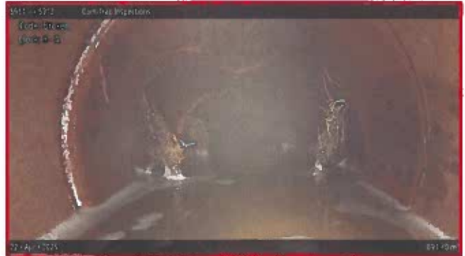
[Grade 4] Broken at 094.80 m, (all clock positions)
