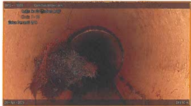
[Grade 3] Roots Medium Joint at 043.50 m, 6 - 9 o'clock
