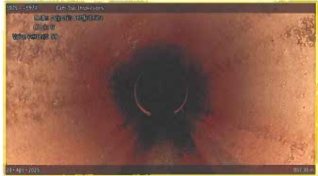
[Grade 2] Deposits Settled Fine (start) at 007.30 m, 6 o'clock
