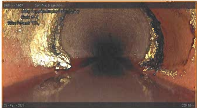
[Grade 3] Deposits Attached Encrustation at 000.10 m, 8 - 4 o'clock
