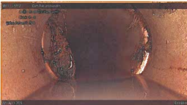
[Grade 3] Roots Medium Joint at 083.60 m, 8 - 4 o'clock
