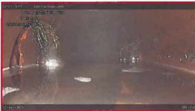
[Grade 4] Roots Medium Barrel at 095.10 m, 8 - 4 o'clock
