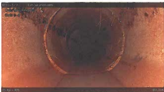
[Grade 1] Roots Fine Joint at 051.70 m, 8 - 4 o'clock
